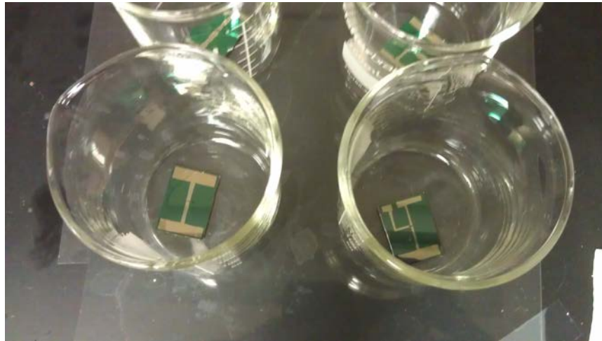
Figure 60: Circuits readied for PBASE functionalization. Recommend actions be performed under a working fumehood as DMF is toxic.
